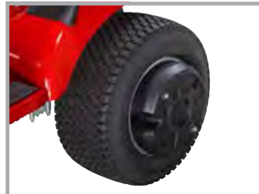
REAR WHEEL WEIGHTS These 33-lb. weights attach easily to provide the extra stability needed when working on slippery ground. Fits SPX™
