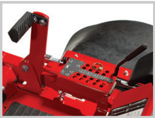
The easy-to-use deck-lift takes the effort out of adjusting cut height. Cutting height ranges from 1.5" - 5" in 0.25" increments.
