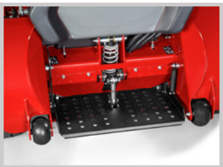
The PTO conveniently disengages when the operator leaves the platform to move an obstacle or pick up debris. When the operator steps back onto the platform and re-engages the PTO switch, the blades start again for continued mowing.
