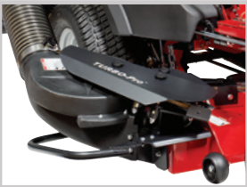
TURBO-Pro Blower* — Length: 31" Height: 16.5" Width: 19" Approximate blower weight: 50 lbs. (44"/48") / 53 lbs. (52") / 55 lbs. (61"), includes mounting bracket
