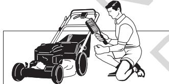
Accumulation of grass and debris can result in a fire. Be sure to clean any accumulation of grass and debris with a brush or compressed air, before and after operation.
