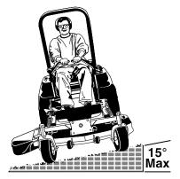
Operation on slopes can be dangerous. Using the unit on a slope that is too steep where you do not have adequate wheel traction (and control) can cause sliding, loss of steering, control, and possible rollover. You should not operate on a slope greater than 15 degrees (a 5.4 foot rise over a 20 foot length).
