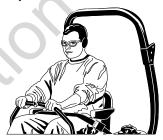
Keep the roll bar in the raised position and fasten the seat belt. There is no roll over protection when the roll bar is down! Do not jump off if the mower tips (it is safer to be secured by the seat belt with the roll bar raised.)
