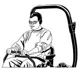
Keep the roll bar in position and fasten the seat belt. Do not jump off if the mower tips (it is safer to be secured by the seat belt.)
