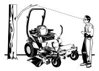
Check for overhead clearances before driving under any objects. Do not allow the roll bar to contact low overhanging obstacles such as tree branches and guide wires.
